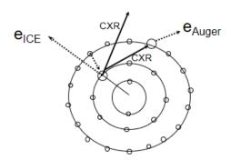
5. As is the case whenever an electron is ejected from an outer orbital, regardless of what caused the ejection, characteristic X-rays and Auger electrons will be produced. From a diagnostic standpoint, Auger electrons are useless and increase the internal radiation dose to the patient. The same can be said of the X-rays, unless their energy is in the imageable range of ~ 70-400 keV, in which case they may be used for imaging.
