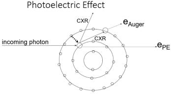
Auger electrons are ejected by the secondary process rather than the primary process
