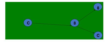
The cue ball hits the 8 ball a glancing blow on the right side, making a partial transfer of energy. The 8 ball is deflected toward upper left and the cue ball is deflected toward the lower right. This is analogous to the partial transfer of energy when a high energy photon ejects an electron in one direction and the deflected photon travels in a different direction.
