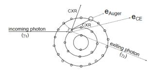
As is evident from the diagram above, the incoming photon transfers part of its energy to the electron (a partially elastic collision) and the electron is ejected. The gamma ray, now lower in energy due to the collision, is deflected at an angle away from the ejected electron. This angle of deflection is referred to as angle  $\phi$  in the equation below:
